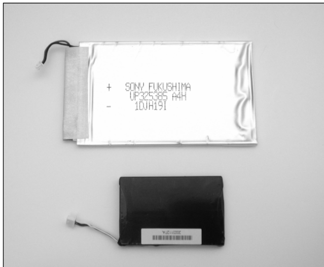
Figure A.15 iPod Batteries: First and Second-Generation (Top) and Third-Generation (Bottom)
