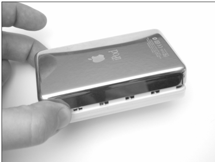
Figure A.23 Reattaching the Metal Half of the Case
