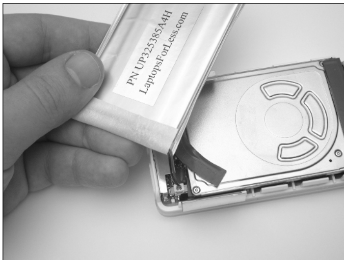
Figure A.20 Connecting the New Battery
