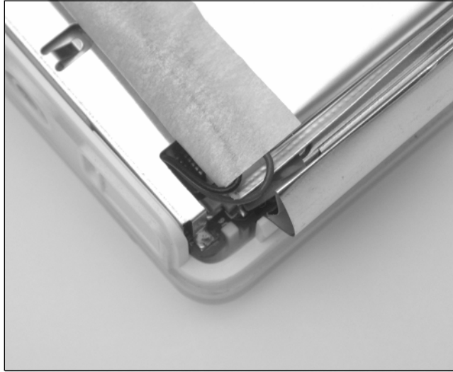
Figure A.22 Power Cable Safely Tucked Away
