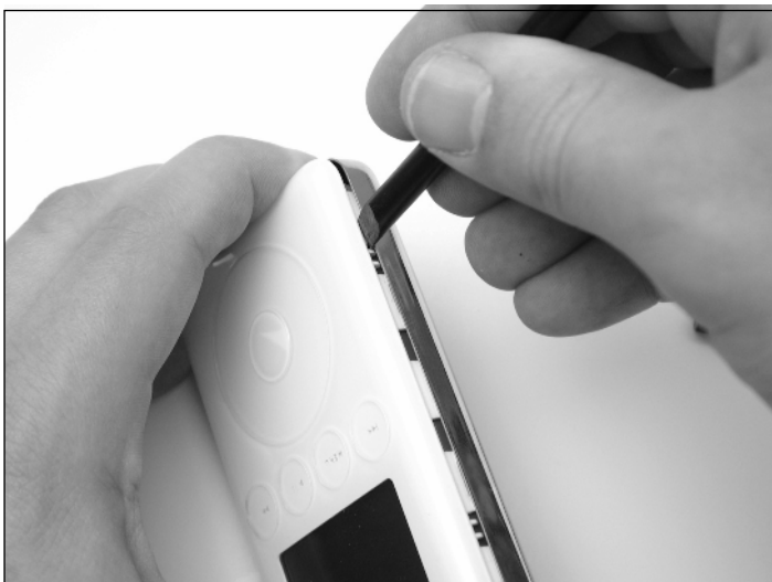
Figure A.12 Unclip all the Tabs
