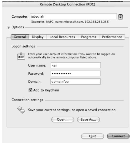
Figure 3.10 Configuring a Remote Desktop Connection to Save as a File
