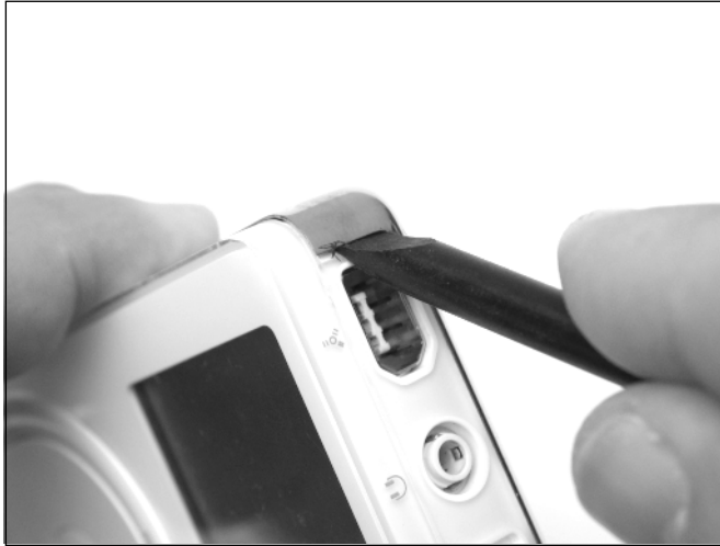
Figure A.6 Start Prying at the Top of the Case
