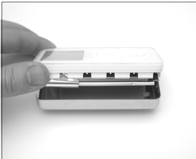
Figure A.9 Lifting Apart the Two Halves of the iPod
