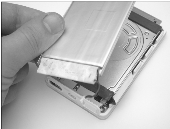
Figure A.19 Removing the Old Battery
