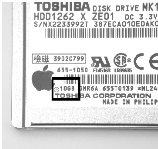
Figure A.38 Drive Capacity printed on the Hard Drive Sticker
