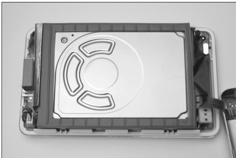
Figure A.34 Hard Drive Back in Place
