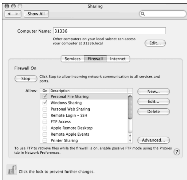
Figure 7.8 Your Firewall can be Enabled with One Button Click
