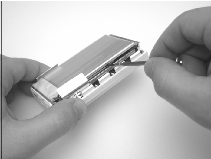
Figure A.18 Prying the Battery from the Rubber Strips
