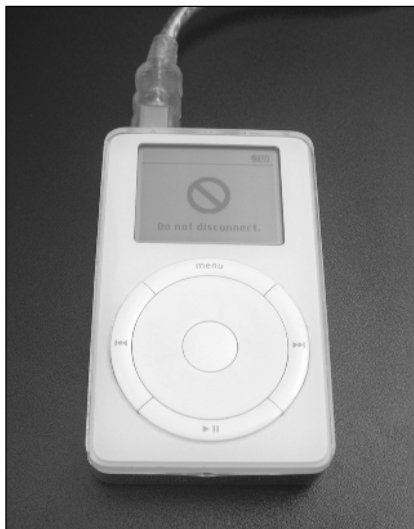
Figure A.24 Charging the New Battery
