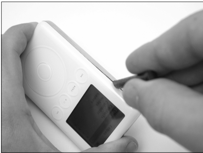
Figure A.10 Prying into the Case
