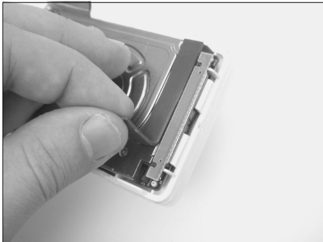
Figure A.42 Removing the Rubber Pads
