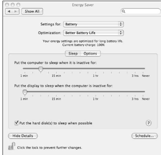
Figure 7.10 The Energy Saver System Preference Pane Has a Number of Tunable Power Options
