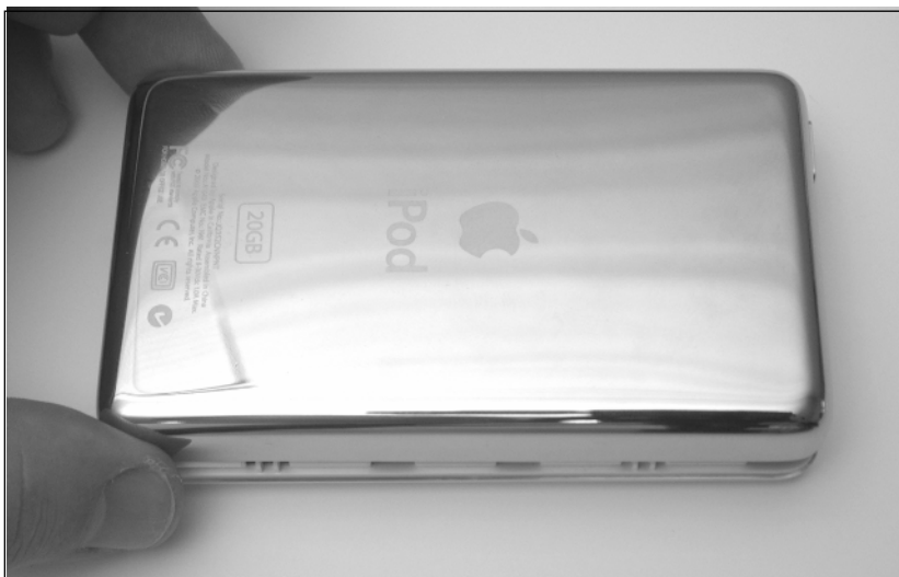
Figure A.35 Snapping the Case Back Together
